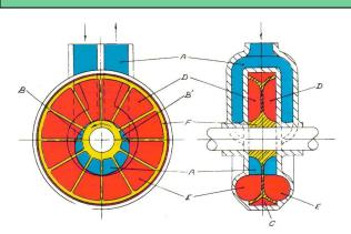
Our patented impeller floats freely in the pump housing cavity which allows it to "conform" to whatever conditions are necessary for maximum efficiency and performance.. \*\* Why? Because our Liquid Ring Pump technology is very different from the competition. We combine the benefits of the turbine, centrifugal and positive displacement pump designs. The Lobee Liquid Ring Pump will pull a high vacuum, deliver clean compressed air and pump non-lubricating liquids.
